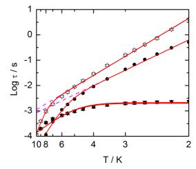
**Fig. 4** Log scale plots of the temperature dependence of the relaxation time for **1(+)** and **1(-)** in up and down triangles and *rac*-**1**·0.5C<sub>6</sub>H<sub>14</sub> in circles. Empty symbols indicate measurements in zero external dc field while full symbols indicate measurements at **1** kOe. Red lines correspond to the best-fitted curves with modified Arrhenius laws (see text). Dashed pink lines are the high temperatures extension of the regime reg<sub>1</sub>.
