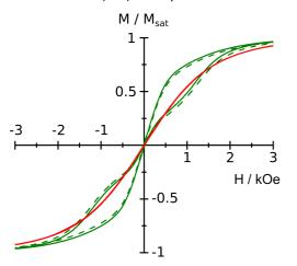
Fig. 5 Magnetic hysteresis loops recorded at 500 mK and measured at a sweep rate of 16 Oe s<sup>-1</sup> for 1(+) (full green line), 1(-) (dashed green line) and rac-1.0.5C<sub>6</sub>H<sub>14</sub> (red line).
