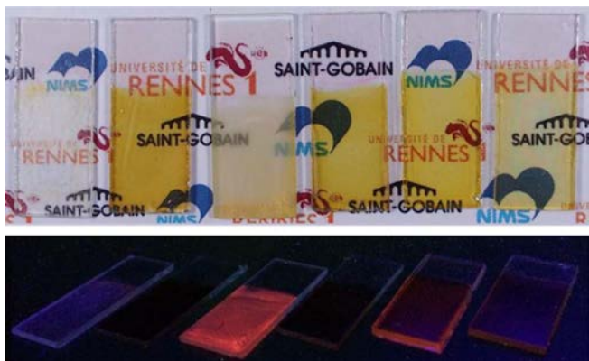
Figure 3. The \text{Mo}_6 cluster thin films deposited from (left to right) water, ethanol, 1-propanol, acetone and MEK solutions at 15 V for 20 s and from acetyl acetone solution at 50 V for 40 s (upper), respectively. Image of the luminescence of the cluster thin films irradiated at 324 nm wavelength (under).
