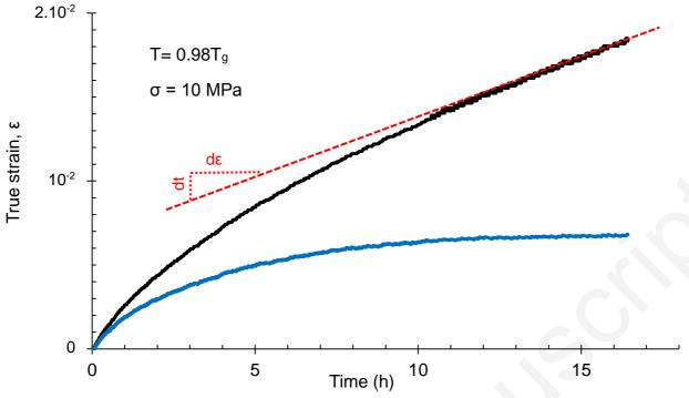
Fig. 11. Compressive creep experiment at  $0.98T_g$  under a 10 MPa load for the  $0.3BaO-0.2TiO_2-0.5SiO_2$  glass composition. The true strain (black) is the sum of the anelastic (or delayed elastic) (blue) and the stationary (viscous) (red) contributions.
