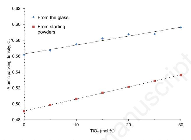
Fig.8. Atomic packing density calculated from the density of the glass Eq. (13) and the density of the starting powders as a function of TiO<sub>2</sub> molar content.
