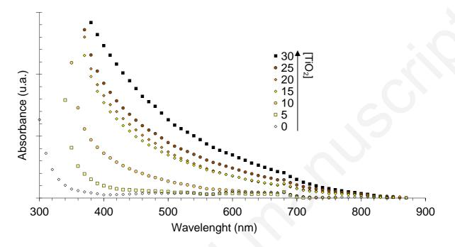
Fig. 2. Absorption spectra for different values of  $x = [TiO_2]$ .
