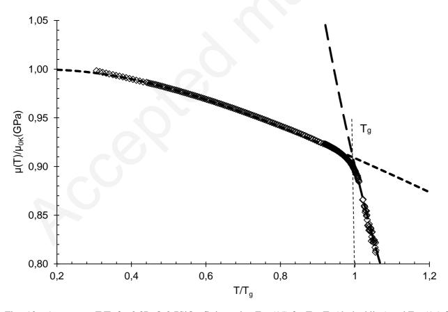
Fig. 10.  $\mu/\mu_{0K}$  versus  $T/T_g$  for 0.3BaO-0.7SiO<sub>2</sub>, fitting using Eq. (15) for  $T < T_g$  (dashed line) and Eq. (16) for  $T > T_g$  (dotted line).
