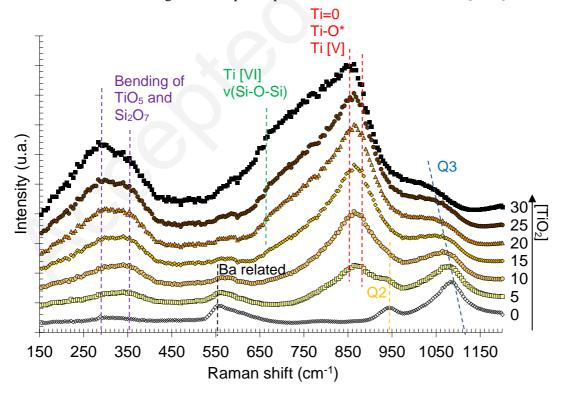
Fig. 3. Raman spectrum for different values of  $x = [TiO_2]$ .
