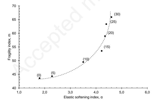
Fig. 14. Fragility index, m, calculated by means of Eq. (23) as a function of the elastic softening index,  $\alpha$ , calculated from Eq. (16) (numbers in brackets indicate the TiO<sub>2</sub> content, in mol.%).
