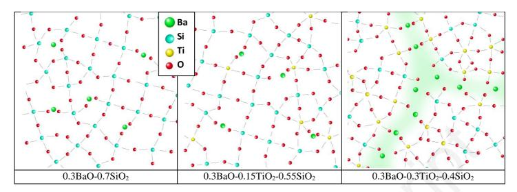
Fig. 4. Schematic drawings of the atomic network for x = 0; 0.15; 0.30 glasses.
