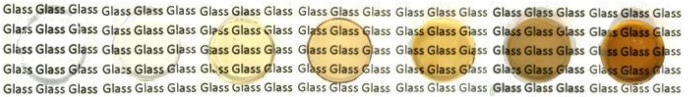
Fig. 1. Comparison of color and transparency of the different glasses, from left to right x = 0; 0.05; 0.10; 0.15; 0.20; 0.25; 0.30 (25 mm diameter and 2 mm thick disks).
