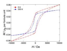
**Figure 8.** Magnetic field dependence of the magnetization of LiNbO<sub>3</sub>-type InFeO<sub>3</sub> at 5 and 300 K.
