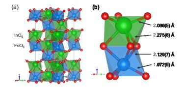
Figure 2. (a) Polyhedral representation of the crystal structure of LiNbO<sub>3</sub>-type InFeO<sub>3</sub> refined against the TOF NPD data at 300 K. Green, blue, and red spheres represent In, Fe, and O atoms, respectively. (b) Local coordination environment of  $InO_6$  and  $FeO_6$ octahedra stacked along the hexagonal c-axis, showing a face-sharing octahedral pair.
