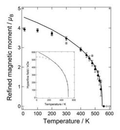
**Figure 9.** Temperature dependence of the magnetic moment of  $LiNbO_3$ -type  $InFeO_3$  refined by TOF NPD at WISH (open circles) and NPD at WOMBAT (solid circles). The solid curve represents the critical law fitting to WOMBAT data. The inset shows the temperature dependence of hyperfine field (open squares) and the critical law fitting (solid line).
