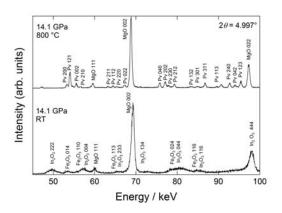
Figure 4. In situ SXRD patterns of InFeO<sub>3</sub> measured by the energy-dispersive method: a pressure of 14.1 GPa was applied to a mixture of  $In_2O_3$  (bixbyite-type) and  $Fe_2O_3$  (corundum-type) at room temperature (lower) and then the temperature was increased to 800 °C (upper). Pv denotes the orthorhombic perovskite. MgO is the pressure maker.
