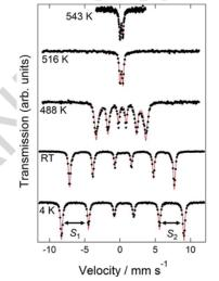
**Figure 5.** <sup>57</sup>Fe Mössbauer spectra of LiNbO<sub>3</sub>-type InFeO<sub>3</sub> at various temperatures. The dots represent the experimental data, and the solid red lines the total fits.  $S_1$  and  $S_2$  denote the relative shifts of the peaks.
