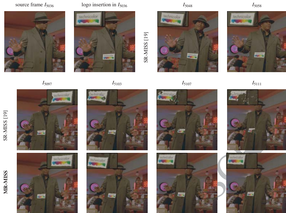
Figure 7: Texture insertion in I_{5036} and propagation along the Hope sequence up to I_{5111} . We compare SR-MISS [19] and the proposed MR-MISS strategy using \{I_{5036}, I_{5063}, I_{5073}\} as reference frames. Both methods use 2D-DE input optical flows from [24].
