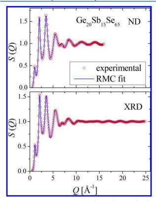
**Figure 3.** ND and XRD structure factors (symbols) and fits (lines) for the final model (see text) of the Ge<sub>20</sub>Sb<sub>15</sub>Se<sub>65</sub> sample.
