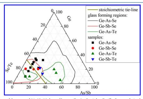
**Figure 6.** Ternary diagram of the compared 14–15–16 glasses. (Squares: Ge–As–Se, circles: Ge–Sb–Se, upward triangle: Ge–As–Te, downward triangle: Ge–Sb–Te.) The glass-forming regions are shown only schematically. The stoichiometric tie-line is also indicated.
