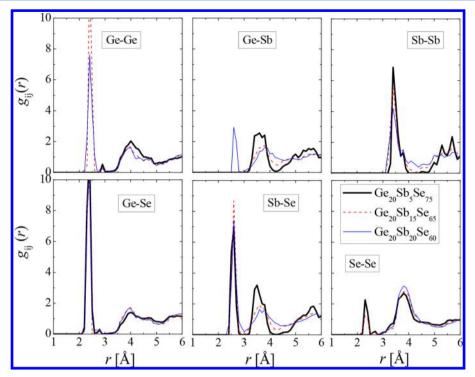
Figure 5. Partial pair correlation functions for the final models (see text) of the Ge–Sb–Se samples. (Thick solid lines:  $Ge_{20}Sb_5Se_{75}$ , dashed lines:  $Ge_{20}Sb_1Se_{65}$ , thin solid lines:  $Ge_{20}Sb_2Se_{60}$  composition.)
