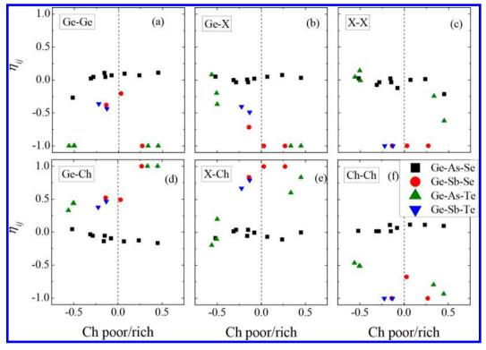
Figure 7.  $\eta_{ij}$  values of the compared glasses. (Squares: Ge–As–Se, circles: Ge–Sb–Se, upward triangle: Ge–As–Te, downward triangle: Ge–Sb–Te.) The compositions are arranged by their chalcogen excess/deficiency (see text). X represents As and Sb atoms, and Ch represents Se and Te atoms. Subfigure (a) shows  $\eta_{\text{GeGe}}$  (b)  $\eta_{\text{GeX}}$  (c)  $\eta_{\text{XX}}$  (d)  $\eta_{\text{GeCh}}$  (e)  $\eta_{\text{XCh}}$ , and (f)  $\eta_{\text{ChCh}}$ .
