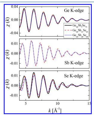
**Figure 2.** Filtered Ge K-edge, Sb K-edge, and Se K-edge EXAFS spectra for the Ge–Sb–Se samples. (Thick solid lines:  $Ge_{20}Sb_5Se_{75}$ , dashed lines:  $Ge_{20}Sb_{15}Se_{65}$ , thin solid lines:  $Ge_{20}Sb_{20}Se_{60}$  composition.)
