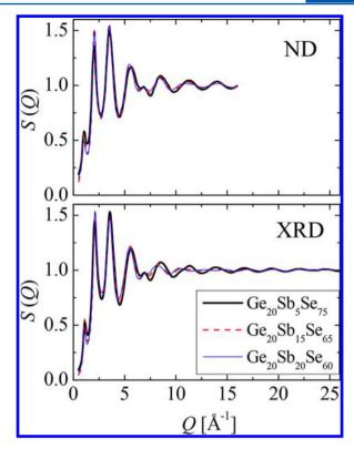
**Figure 1.** ND and XRD structure factors for the Ge–Sb–Se samples. (Thick solid lines:  $Ge_{20}Sb_5Se_{75}$ , dashed lines:  $Ge_{20}Sb_{15}Se_{65}$ , thin solid lines:  $Ge_{20}Sb_{20}Se_{60}$  composition.)
