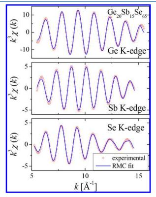
Figure 4.  $k^3$ -weighted, filtered EXAFS spectra (symbols) and fits (lines) for the final model (see text) of the  $Ge_{20}Sb_{15}Se_{65}$  sample.
