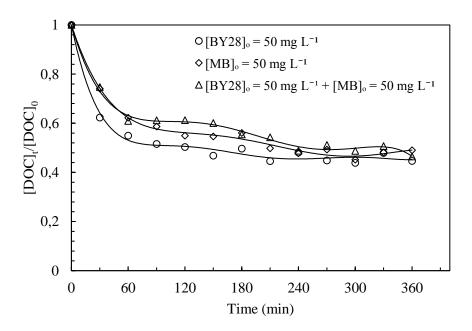
**Figure 6.** Time-courses of mineralization during the electrochemical pretreatment under the optimal conditions for Methylene Blue, Basic Yellow 28 and the dyes mixture E=2.4 V/SCE,  $T=25 \,^{\circ}\text{C}$ ,  $\omega=600 \text{ rpm}$  and pH=2
