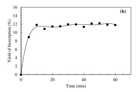
**Figure 7.** (a):Time-courses of  $[COD]_t/[COD]_0$  values during activated sludge culture of the dyes mixture pretreated during 6 h ( $\Diamond$ ). (b) Biosorption on activated sludge of intermediate compounds formed after the electrochemical oxidation of the dyes mixture ( $\circ$ ).
