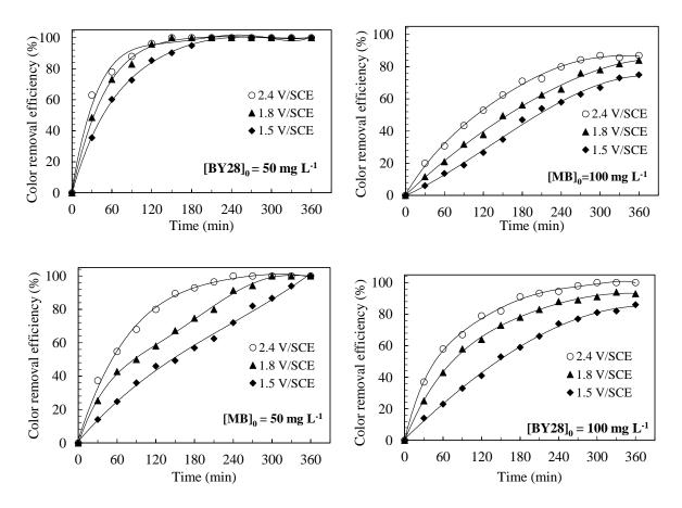
**Figure 3.** Influence of the working potential on Methylene Blue and Basic Yellow 28 degradationT= 25 °C,  $\omega$  = 600 rpm and pH 2
