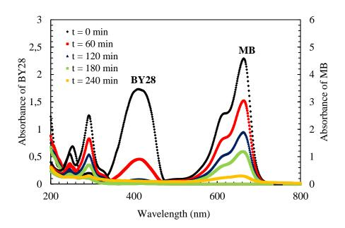
**Figure 5**. Absorbance spectra of BY28 and MB recorded before the electrochemical pretreatment and after different electrolysis times in the optimized conditions:  $[BY28]_0 = 50$  mg L<sup>-1</sup>,  $[MB]_0 = 50$  mg L<sup>-1</sup> E= 2.4 V/SCE, T= 25 °C,  $\omega = 600$  rpm and pH 2
