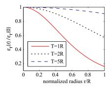
Fig. 4. Relative permittivity distribution of a dielectric Mikaelian lens as a function of the normalized radius: influence of of the ratio thickness over radius of the lens T/R.
