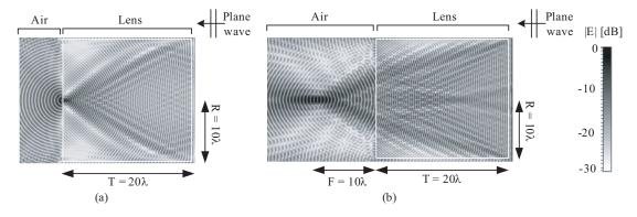
Fig. 3. Near electric field mappings computed by CST Microwave Studio of a plane wave impinging on (a) a Mikaelian lens and (b) a generalized Mikaelian lens. The white square shows the location of the lens.
