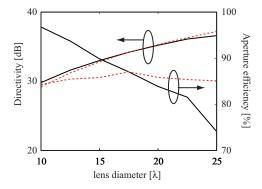
Fig. 5. Directivity and aperture efficiency as a function of the lens diameter for the ideal Mikaelian (solid line) and Luneburg (dashed line) lens fed by a circular waveguide.
