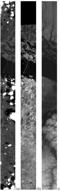
Fig. 4. Registered Hyperion band #25 (a), Landsat 8 band B1 (b) and DEM (c). Gray levels ranging from black to white cover intensity ranges 1100...3800 for Hyperion, 8500...9600 for Landsat 8 and 50...250m for DEM. Images size is 256 by 3129 pixels.
