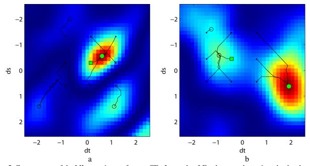
Fig. 5. Convergence of the  $ML_{fBm}$  estimator for two CFs. Larger log-LF values are shown in red color, lower – in blue color. Nine convergence paths are shown in black; the starting points are marked as "•", the end points - as "o"; the point  $(\Delta t_0, \Delta s_0)$  - as green " $\Box$ " marker; the global log-LF maximum - as green "o" marker. Initial guess is within (a) and outside (b) the mail lobe of the log-LF.
