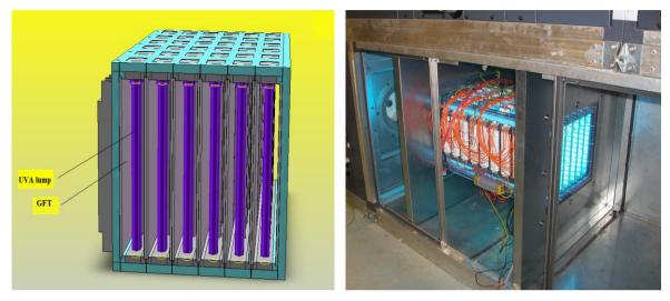
Fig. 4: A schematic representation and photo of photocatalytic system used in pilot unit
