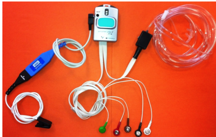
Figure 2: The prototype cardiorespiratory Holter device with associated sensors (ECG electrodes, SaO 2 ear sensor and nasal pressure cannula).
