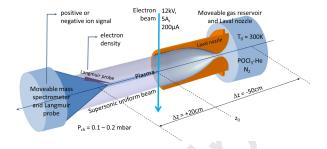
Figure 1: Supersonic cold uniform beam in the CRESU apparatus at Rennes.
