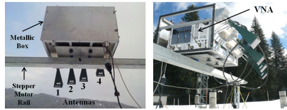
Fig. 1. GB-SAR system of the SAPHIR team of the University of Rennes-1.
