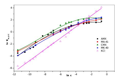
**Fig. 4.** Logarithm of membrane conductivity vs. logarithm of electrolyte concentration (KCl solutions).
