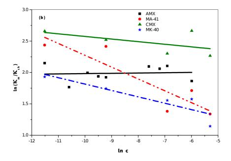
Fig. 7. a) Logarithm of membrane conductivity to solution conductivity ratio vs. logarithm of KCl solution concentration b) Enlargement for very low concentrations  $(10^{-5} - 5 \times 10^{-3} \text{ M})$ .
