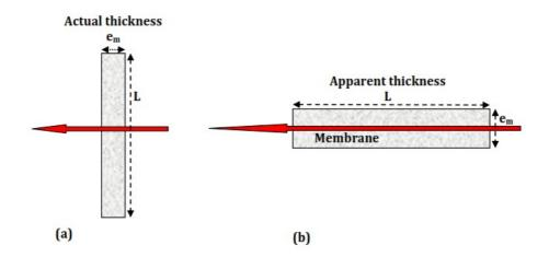
**Fig. 3.** Effective membrane thickness for the different cell configurations. a) actual thickness e<sub>m</sub> in the case of normal measurements, b) apparent thickness L (corresponding actually to the sample length) in the case of lateral measurements (this configuration was used in the present work).
