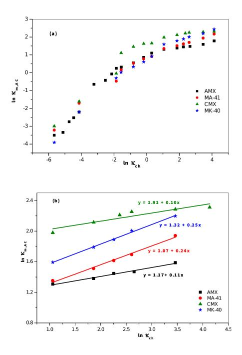
Fig. 6. a) Logarithm of membrane conductivity vs. logarithm of KCl solution conductivity. b) Linear variations obtained for ~0.5  $c_{iso} < \sim 10 c_{iso}$ .
