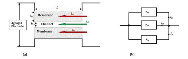
**Fig. 2.** (a) Different electrical current paths through the measuring cell; (b) equivalent electrical circuit;  $i_m$  is the electrical current flowing through each membrane sample,  $i_{ch}$  is the electrical current flowing between membranes,  $r_m$  is the membrane electrical resistance and  $r_{ch}$  solution-filled channel resistance.
