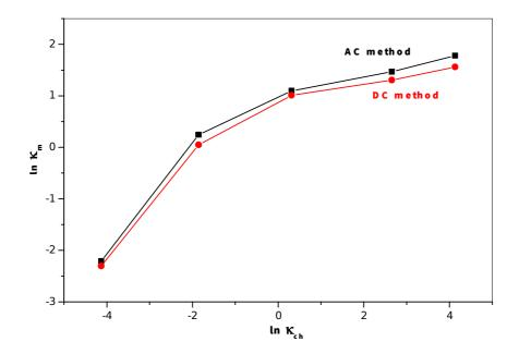
**Fig.8.** Logarithm of the AMX membrane conductivity determined from DC and AC methods vs. logarithm of the KCl solution conductivity.
