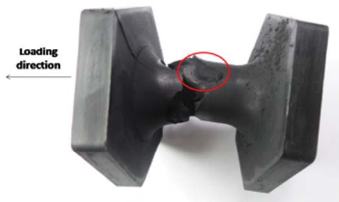
Fig. 8: Ruptured dry specimen.
