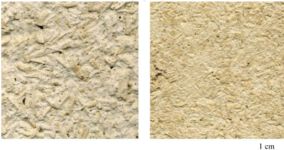
Fig. 2: Picture of specimens: Chanvribat hemp-lime plaster (left) and Terrachanvre hemp-lime plaster (right).
