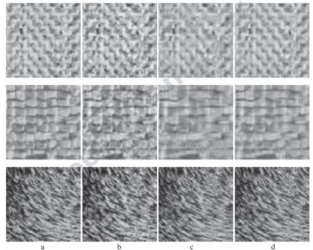
Fig. 16. Fragments of the test images ## 4, 8, and 9: a – original image, b – noisy image with  $\sigma_0^2 = 225$ , c – filtered image by DCT-based filter, d – filtered image by BM3D
