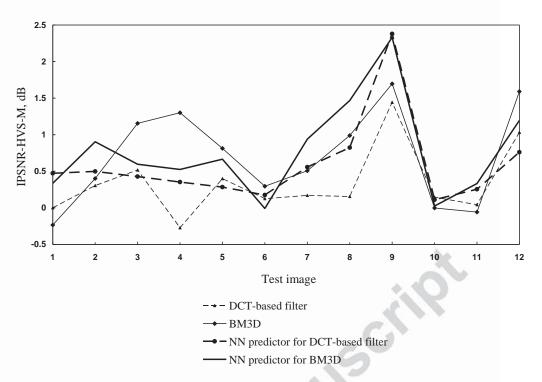
Fig. 14. IPSNR - HVS - M metric and predicted values for spatially correlated noise with  $\sigma_0^2 = 100$
