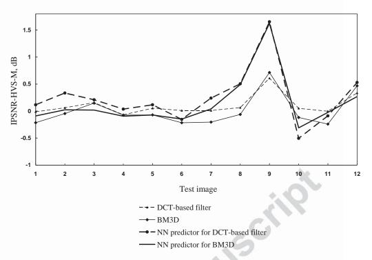
Fig. 13. IPSNR-HVS-M metric and predicted values for spatially correlated noise with  $\sigma_0^2=25$ .
