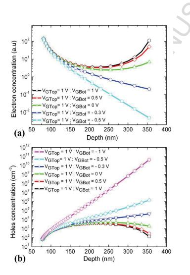
Fig. 9. Simulated distribution of electrons (a) at  $V_{Top}=1V$  ( $V_{GBot}=-0.5$  to 1V) and holes (b) through a 300 nm width nanowire. Bottom channel conduction is as important as top channel's for positive bottom gate biasing.
