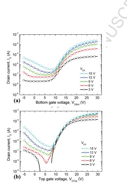
Fig. 3. Transfer characteristics of poly-Si NWFET  $I_{DS}$ - $V_{GS}$ : (a) bottom-gate and (b) top-gate transistors (1000 nanowires, L=5  $\mu$ m), showing an N-type enhancement and different off-current behavior.
