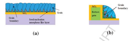
Fig. 4. Schematic cross section view illustrating the columnar type structure of a polycristalline silicon layer (a). Size lowering leads to a higher defects density within the polycristalline SiNWs close to the Si nanostructure/SiO<sub>2</sub> interface (b)
