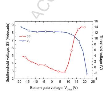
Fig. 7. Bottom-gate bias effect on subthreshold slope and threshold voltage on poly-SiNWs FET with separated top and bottom-gate electrodes ( $V_{DS} = 3 \text{ V}$ ). A relative stability of device is observed for  $V_{GBot} < 10 \text{ V}$ .
