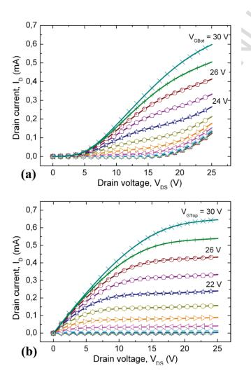
Fig. 5. Output characteristics of poly-Si NWFET  $I_D$ - $V_{DS}$ : (a) bottom-gate and (b) top-gate transistors (1000 nanowires, L=5  $\mu$ m). Measurement step is 2V. Saturation mode is easily reached for TGT and is not reached for BGT.
