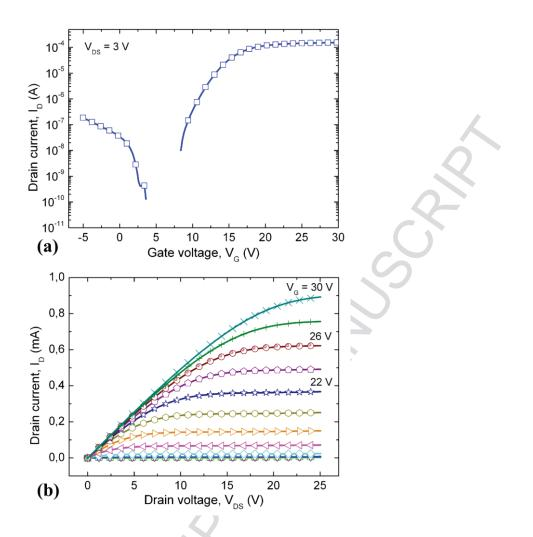
Fig. 10. Gate-All-Around poly-Si NWFET transfer  $I_D$ -V<sub>G</sub> (a) and output  $I_D$ -V<sub>DS</sub> (b) characteristics, showing a typical N-type FET behavior.
