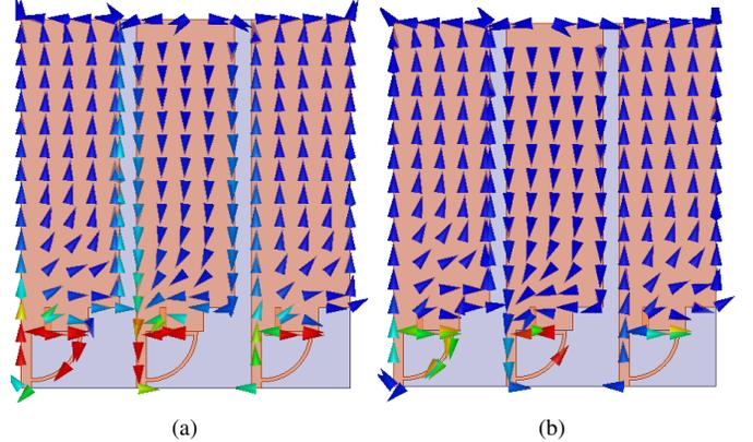
Fig. 23. Three-element array mounted on a PCB's simulated surface current distribution. (a) Fully-driven array and (b) parasitic one.
