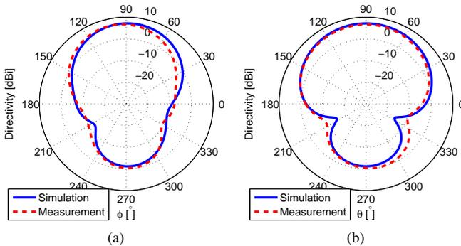
Fig. 25. Two-element array mounted on a PCB's measured 2D total directivity radiation patterns. (a) Horizontal plane and (b) vertical plane.
