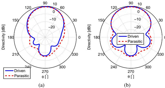
Fig. 21. Three-element array mounted on a PCB's simulated 2D total directivity radiation patterns. (a) Horizontal plane and (b) vertical plane.
