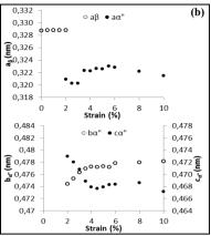
Fig. 3. a) Evolution of lattice parameters of B2, R and B19' phases as a function of the applied strain during in situ tensile tests for NiTi. b) Evolution of lattice parameters of  $\beta$  and  $\alpha$ " phases for Ti-27Nb.
