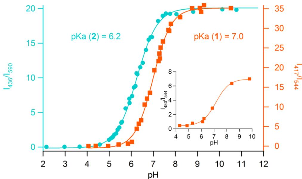
**Fig. 4** Determination of pKa values of compound **1** (orange) and **2** (cyan) under 1P excitation at 380 nm and 386 nm, respectively. Inset: ratiometric behavior of **1** under 2P excitation at 750 nm.
