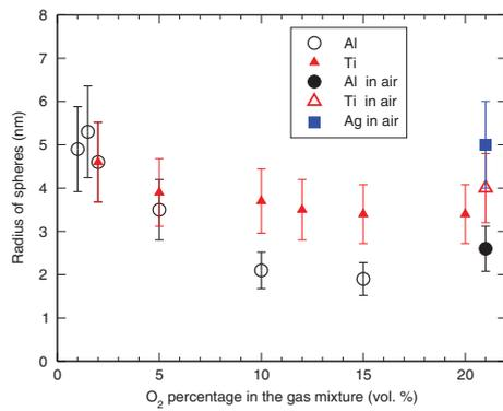
Figure 3: Variation of the mean radius of nanoparticle spheres,  $R$ , determined by SAXS experiments as a function of the  $O_2$  percentage in the  $O_2-N_2$  gas mixture for Al and Ti targets. The values of  $R$  obtained in the case of laser treatments of Al, Ti and Ag targets in air are also shown.
