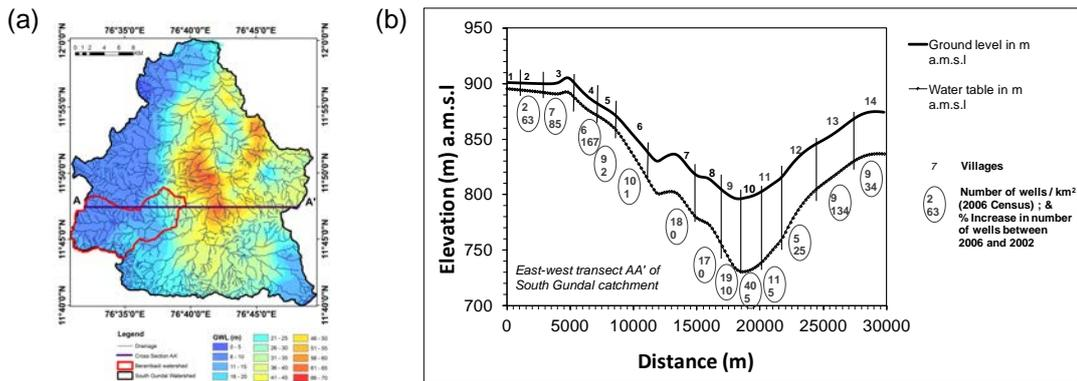
**Fig. 1** Illustration of data acquisition in the South Gundal watershed: (a) stream drainage and depth to groundwater levels (obtained using about 600 disused bore wells); (b) topographic elevation (in m a.m.s.l.) and water table level along the transect AA'.
