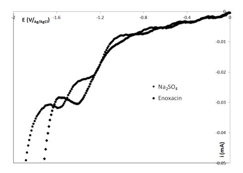
**Supplementary material 1:** Current-potential curves obtained by cyclic voltammetry with a vitreous carbon electrode ( $S=3.14~\text{mm}^2$ ),  $r=20~\text{mV.s}^{-1}$ , under nitrogen atmosphere and T=298~K, in  $Na_2SO_4~0.05~\text{mol.L}^{-1}$  at pH 3.
