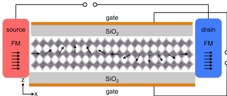
Figure 6: Scheme of a sFET as proposed by Datta and Das<sup>72</sup> based on hybrid organic-inorganic perovskites with a representation of the spin precession from the source to the drain.
