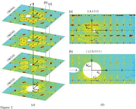
(a) Reconstructed reciprocal planes  $(\mathbf{a}^*, \mathbf{b}^*)$  for m = 1, 2, 3 and 4 measured by X-ray diffraction at 10 K on *n*-nonadecane–urea. (b) Reconstructed reciprocal planes  $(\mathbf{b}^*, \mathbf{c}^*)$  for h = 1 and h = 1/2 (dashed lines in the left figure).
