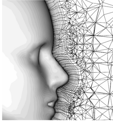
Figure 5: Detail of the virtual thermal manikin, 500000 cells [125]
