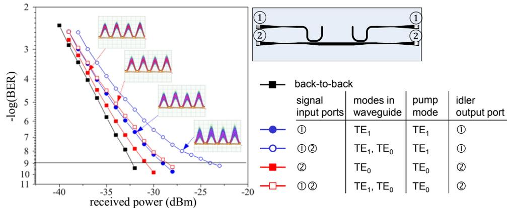
Fig. 3. BER characterization of mode-selective wavelength conversion.
