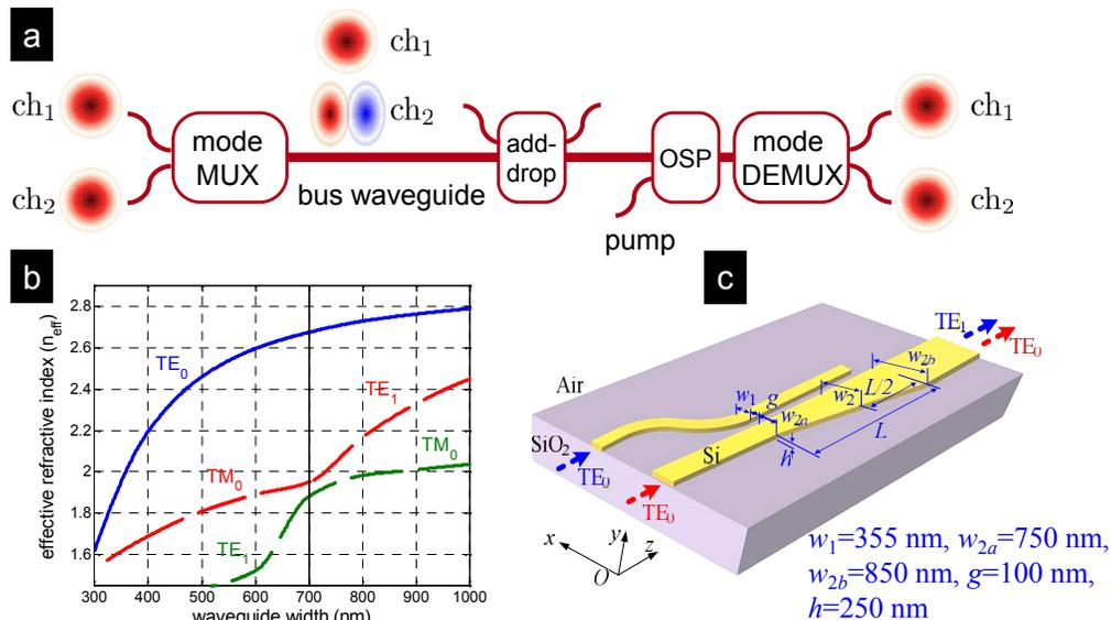
Fig. 1. (a) Principle of an on-chip mode-multiplexed system. (b) Effective indices of the TE<sub>0</sub>, TE<sub>1</sub> and TM<sub>0</sub> modes of an air-clad SOI waveguide of height  $h = 250$  nm as a function of the waveguide width. (c) Layout of a TE<sub>0</sub> and TE<sub>1</sub> mode (de)multiplexer based on a tapered asymmetric directional coupler.
