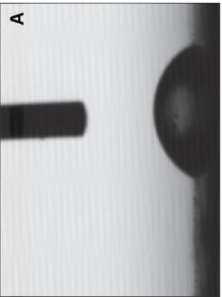
Figure 2. Shape of liquid drop on (A) compact, and (B) porous Ti20Mo alloys after 1 day exposure to aerated 3 wt.% NaCl solution.
