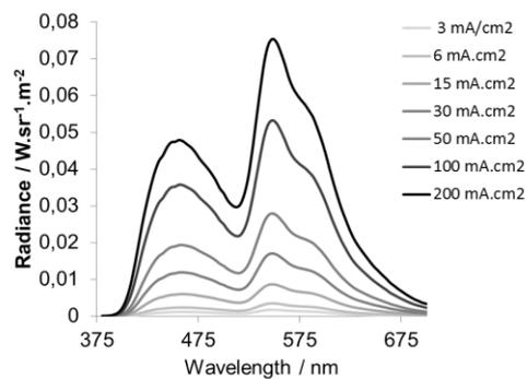
**Figure 8.** Effect of current density on the electroluminescence of device **D**.
