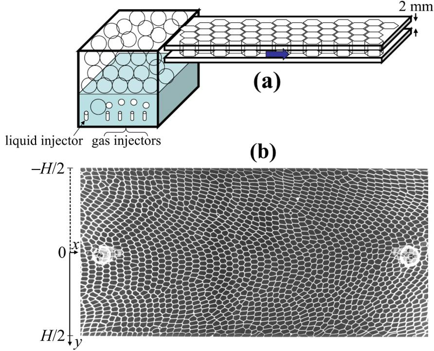
FIGURE 1. (a) Sketch of the side view of the setup. (b) Snapshot of an experiment. The distance between the two side walls is  $H = 106.6$  mm. The average bubble size is  $12.3$  mm<sup>2</sup> and the liquid fraction is  $\phi_l = 4.8\%$ . The two spots at the left and right of the image are the points between which the pressure drop is measured.
