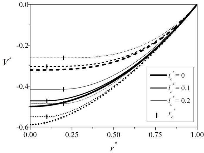
Figure 4: Velocity profile for nonlocal viscous fluids ( $\tau_0^* = 0.25$ ) with  $l_c^*$  ranging from 0 to 0.2 for Power law fluid with  $n = 0.5$  (dashed lines), Power law fluid with  $n = 1.5$  (dotted lines) and Newtonian fluid (solid lines).
