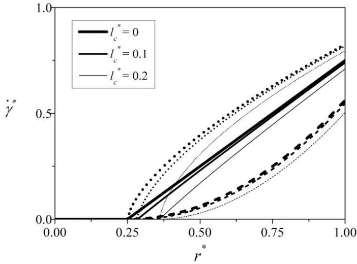
Figure 1: Shear rate profile for nonlocal viscoplastic fluids ( $\tau_0^* = 0.25$ ) with  $l_c^*$  ranging from 0 to 0.2 for Herschel-Bulkley fluid with  $n = 0.5$  (dashed lines), Herschel-Bulkley fluid with  $n = 1.5$  (dotted lines) and Bingham fluid (solid lines).
