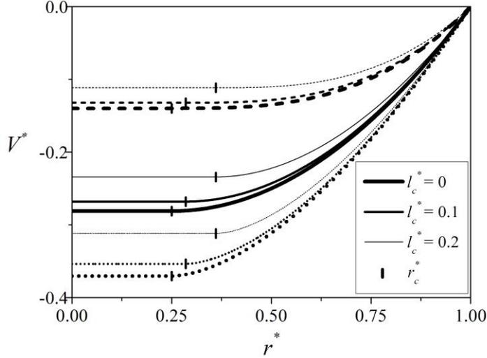
Figure 3: Velocity profile for nonlocal viscoplastic fluids ( $\tau_0^* = 0.25$ ) with  $l_c^*$  ranging from 0 to 0.2 for Herschel-Bulkley fluid with  $n = 0.5$  (dashed lines), Herschel-Bulkley fluid with  $n = 1.5$  (dotted lines) and Bingham fluid (solid lines).
