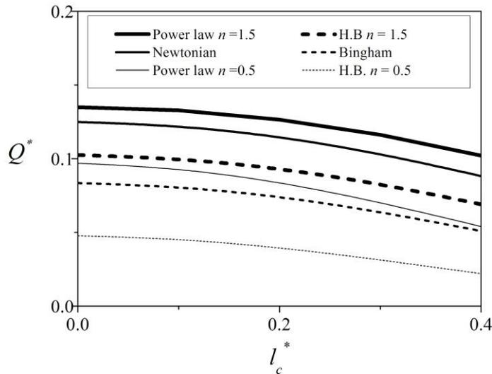
Figure 5: Dimensionless flow rate vs. dimensionless characteristic length for nonlocal viscous fluids (solid lines) and viscoplastic fluids with  $\tau_0^* = 0.25$  (dashed lines) for  $l_c^*$  ranging from 0 to 0.4 (H.B. signifies Herschel-Bulkley).
