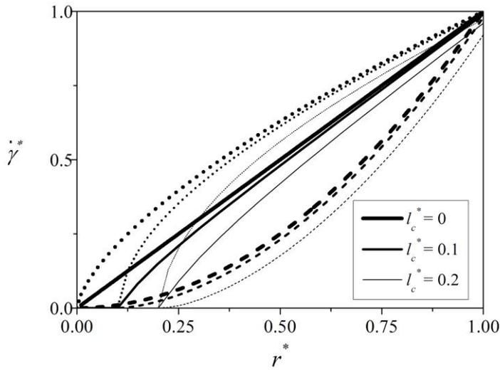
Figure 2: Shear rate profile for nonlocal viscous fluids ( $\tau_0^* = 0.25$ ) with  $l_c^*$  ranging from 0 to 0.2 for Power law fluid with  $n = 0.5$  (dashed lines), Power law fluid with  $n = 1.5$  (dotted lines) and Newtonian fluid (solid lines).
