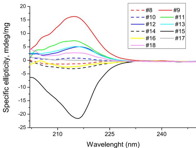
**Fig. 1** Solid state circular dichroism of 11 individual crops of  $\gamma$ -glycine obtained under intensive stirring.
