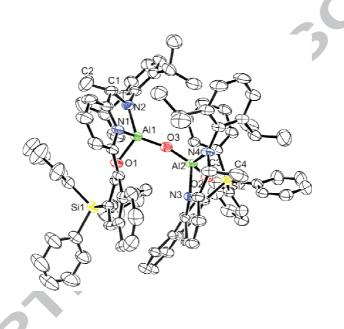
**Figure 7**. Solid-state molecular structure of **3e**<sup>\*\*</sup> (thermal ellipsoids drawn at 50% probability; all hydrogen atoms are omitted for clarity). Selected bond distances (Å) and angles (deg): Al(1)–O(1), 1.7794(15); Al(1)–N(1), 1.9318(17); Al(1)–N(2), 1.817(2); N(2)–C(1), 1.473(3); Al(1)–O(3), 1.690(2); N(1)–Al(1)–N(2), 86.52(8); O(1)–Al(1)–N(1), 89.15(7); Al(1)–N(2)–C(1), 115.64(14); N(2)–C(1)–C(2), 112.6(2); O(1)–Al(1)–N(2), 124.66(8), Al(1)–O(3)–Al(2), 154.80(9).
