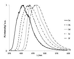
Figure 2. Normalized emission spectra of 3a, b, d, e, f recorded in dichloromethane (5.10<sup>-6</sup> M).
