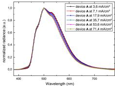
Figure 4. EL emission spectra of the diode A at different current densities
