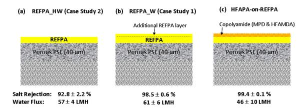
**Figure 5**. Expected structures of RO membranes made by three different processes and their desalination performance (a) REFPA made by the process shown in the case study 2 (w/additional hexane rinse), (b) REFPA made by the process shown in the case study 1, and (c) polyamide bilayer membrane made by the SIP process shown in Figure 1.
