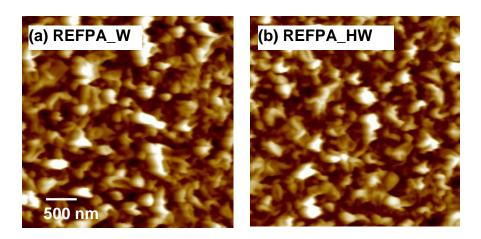
**Figure S2**: AFM topographic images of (a) REFPA\_W and (b) REFPA\_HW; Surface roughness values for REFPA\_W and REFPA\_HW are  $61 \pm 3$  nm and  $60 \pm 4$  nm, respectively.
