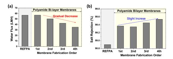
**Figure 2.** Water flux (a) and salt rejection (b) of REFPA and four coupons of polyamide bilayer membranes ( $1^{st} \sim 4^{th}$ ) prepared by sequential interfacial polymerization in the manner of serial membrane dipping.
