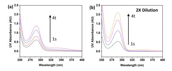
**Figure 4**. Plots showing UV absorption intensities of water samples collected from (a) case study 1 and (b) case study 2. The water samples for case study 2 were diluted two times to avoid saturation of UV signals.
