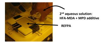
**Figure 6**. A photograph showing a frame process to form polyamide bilayer membranes featuring HFAPA top-layer (copolymerization of HFAMDA and MPD additive) on a REFPA under-layer without cross-contamination
