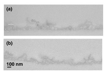
**Figure S1**. Cross-sectional TEM images of (a) REFPA and (b) HFAPA-on-REFPA membranes. The first sample coupon of HFAPA-on-REFPA was used for TEM analysis.
