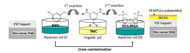
**Figure 1.** A schematic drawing showing a cross-contamination issue in the sequential interfacial polymerization (SIP) process based on the subsequent membrane dipping.
