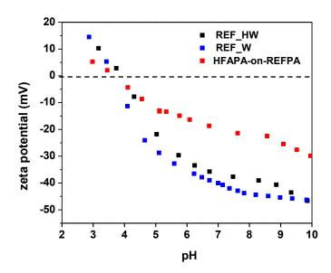
**Figure S3**: pH-dependant zeta-potential curves of REF\_W (blue, prepared by Case Study 1), REF\_HW (Black, prepared by Case Study 2), and HFAPA-on-REFPA (Red, prepared by the scheme in Figure 2). All experiments were performed in a millimolar KCl solution
