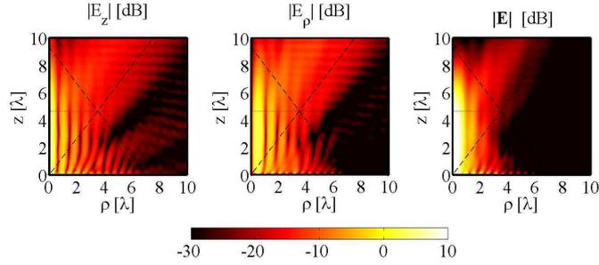
Fig. 7. Electric field radiated by the launcher prototype in Fig. 6, calculated using COMSOL Multiphysics. From left to right,  $|E_z|$ ,  $|E_\rho|$  and  $|E|$ . The axes are normalized with respect to the wavelength ( $\lambda$ ) at the operating frequency  $f$ . The dashed line marks the GO boundaries and the dotted line refers to the field scan shown in Fig. 8.
