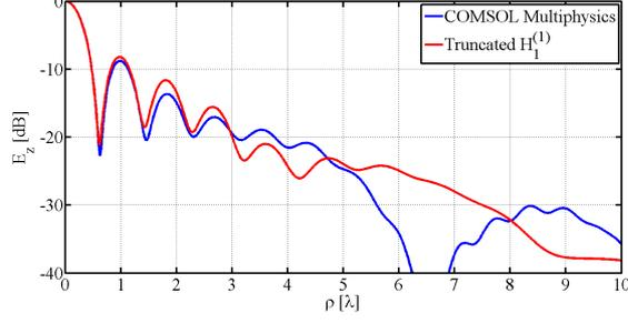
Fig. 8. Normalized  $|E_z|$  component of the electric field at  $z = 4.667\lambda$  for the structure in Fig. 6 simulated with COMSOL Multiphysics. The field radiated by a truncated inward Hankel distribution is shown for comparison.
