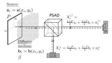
**FIGURE 1.** A generic schematic of the image formation model. A polarization-splitting analyzing device (PSAD) produces two simultaneous images of a partially polarized light source through a turbid medium [12].
