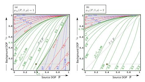
**FIGURE 2.** The contour plots show the range of minimal values of  $\rho$  as a function of P and  $\beta$  for which a specified gain can be achieved, in case of negligible detector noise [12].
