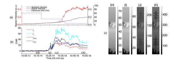
**FIGURE 4.** The evolution of ambient intensity, signal intensity and auto-exposure response is shown in [a] while the evolution of CNR obtained from each representation is shown in [b]. [c] shows a few raw images for the time stamps that are labeled in [b]. [13]
