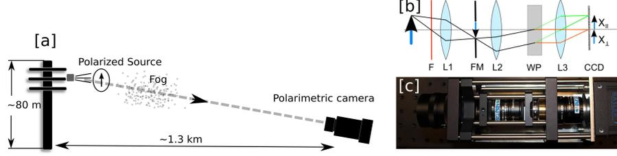
**FIGURE 3.** [a] The schematic shows the long distance polarimetric imaging setup through fog. The principle of the Wollaston-based snapshot polarimetric camera is shown in [b] accompanied with a picture of the actual arrangement in [c].
