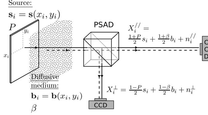
**FIGURE 1.** A generic schematic of the image formation model. A polarization-splitting analyzing device (PSAD) produces two simultaneous images of a partially polarized light source through a turbid medium [12].
