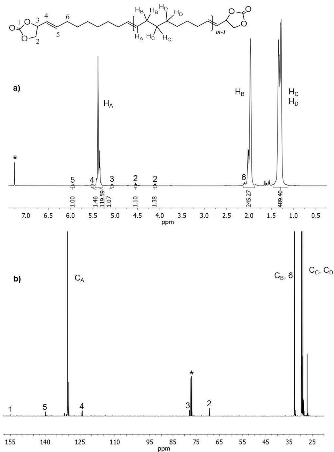
**Figure 1.**  $^1H$  NMR (a, top) and  $^{13}C\{^1H\}$  (b, bottom) NMR spectra (400 and 100 MHz,  $CDCl_3$ , 298 K) of an  $\alpha,\omega$ -di(GC)-PCOE synthesized from the ROMP of COE mediated by **G2** catalyst in the presence of **1** as CTA (Table 1, entry 1) (\* stands for residual solvent resonances).
