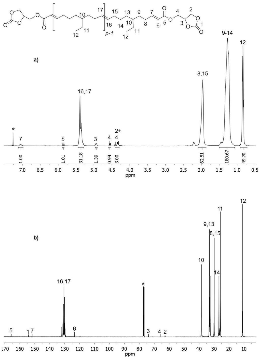
**Figure 4.**  $^1\text{H}$  NMR (top) and  $^{13}\text{C}\{^1\text{H}\}$  NMR (bottom) spectra (400 MHz and 100 MHz,  $\text{CDCl}_3$ , 298 K) of an  $\alpha,\omega$ -di(GC)-P(5-Et-COE) synthesized from the ROMP of 5-Et-COE in the presence of **2** as CTA (Table 1, entry 17; \* stands for residual solvent resonances).
