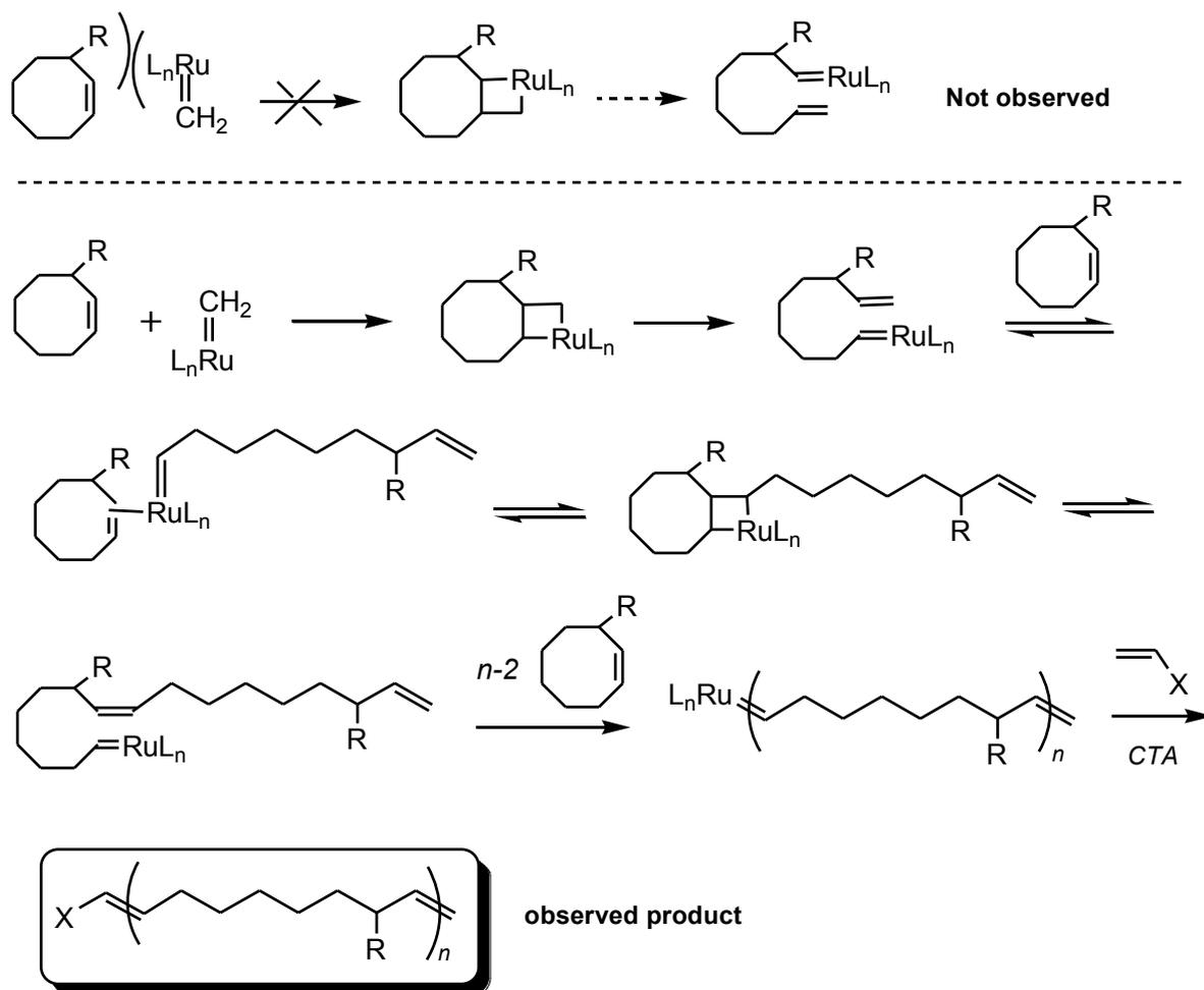
**Scheme 4.** Proposed selectivity model for the ROMP of 3-alkyl-substituted COEs mediated by Grubbs' 2<sup>nd</sup>-generation catalyst.
