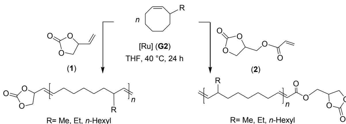
**Scheme 3.** Synthesis of  $\alpha$ -vinyl, $\omega$ -**GC**-P(3-R-COE)s from the ROMP of 3-alkyl-substituted COEs using Grubbs' 2<sup>nd</sup>-generation catalyst (**G2**) and **1** or **2** as CTA.
