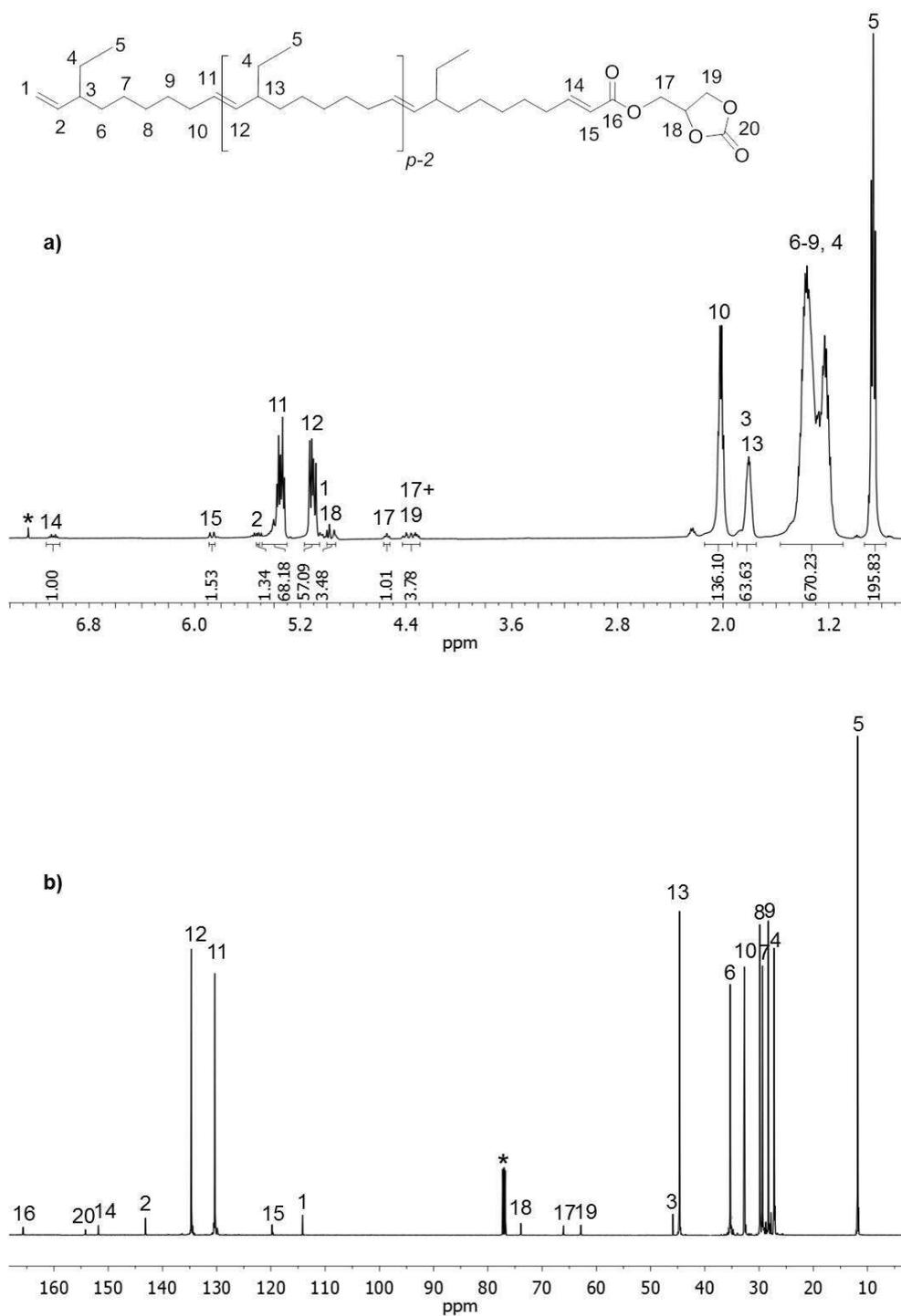
**Figure 3.**  $^1\text{H}$  NMR (a, top) and  $^{13}\text{C}\{^1\text{H}\}$  NMR (b, bottom) spectra (400 and 100 MHz,  $\text{CDCl}_3$ , 298 K) of an  $\alpha$ -vinyl, $\omega$ -GC-P(3-Et-COE) synthesized from the ROMP of 3-Et-COE in the presence of **2** as CTA (Table 1, entry 9) (\* stands for residual solvent resonances).
