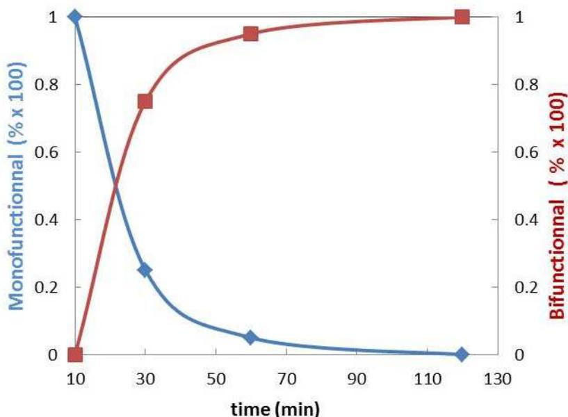
**Figure 2.**  $^1\text{H}$  NMR monitoring of the formation of  $\alpha$ -vinyl, $\omega$ -GC-PCOE (monofunctional,  $\blacklozenge$ ) and  $\alpha,\omega$ -di(GC)-PCOE (bifunctional,  $\blacksquare$ ) during the ROMP of COE promoted by G2 catalyst in the presence of **2** as CTA (Table 1, entry 3).
