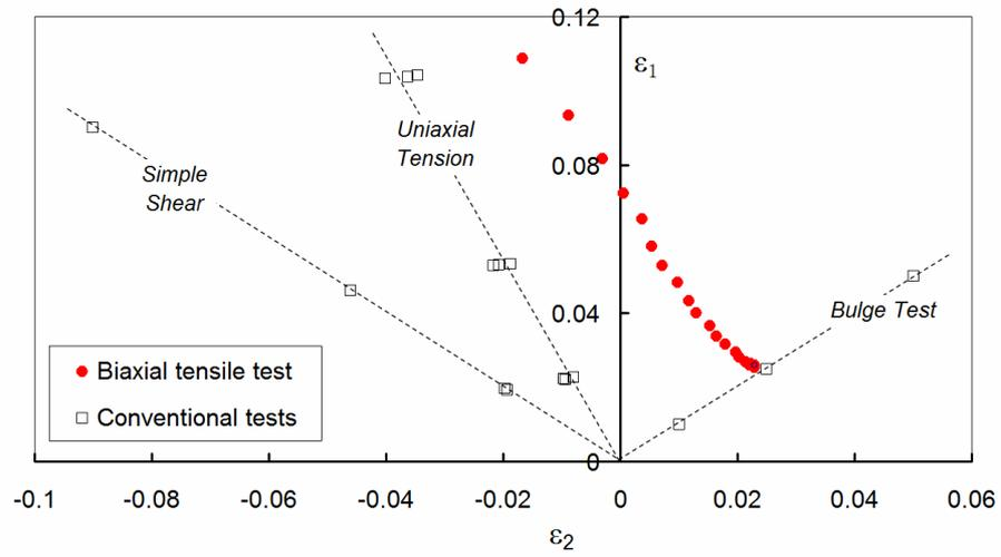
Fig. 17 Strain paths for the two identification methods
