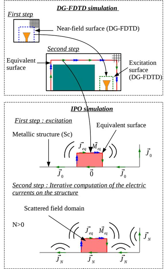
Fig. 3. DG-FDTD/IPO decomposition of the complete scenario.
