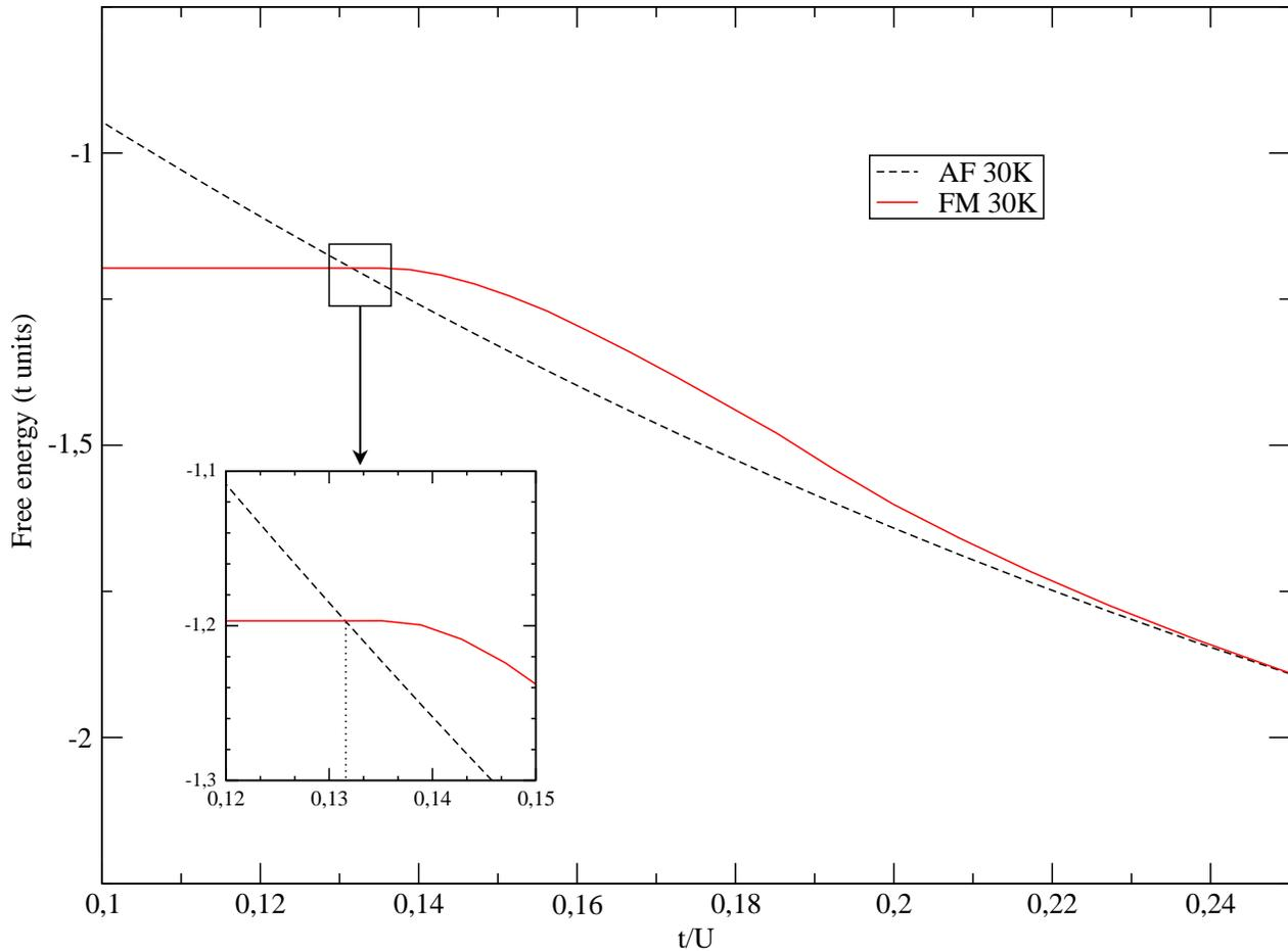
FIG. 4: A phase transition occurs where magnetic-energy curves cross each other. For  $n=0.8$  the system becomes ferromagnetic below  $t/U = 0.13$ . We have chosen an inverse temperature  $\beta \sim 0.003$  eV.
