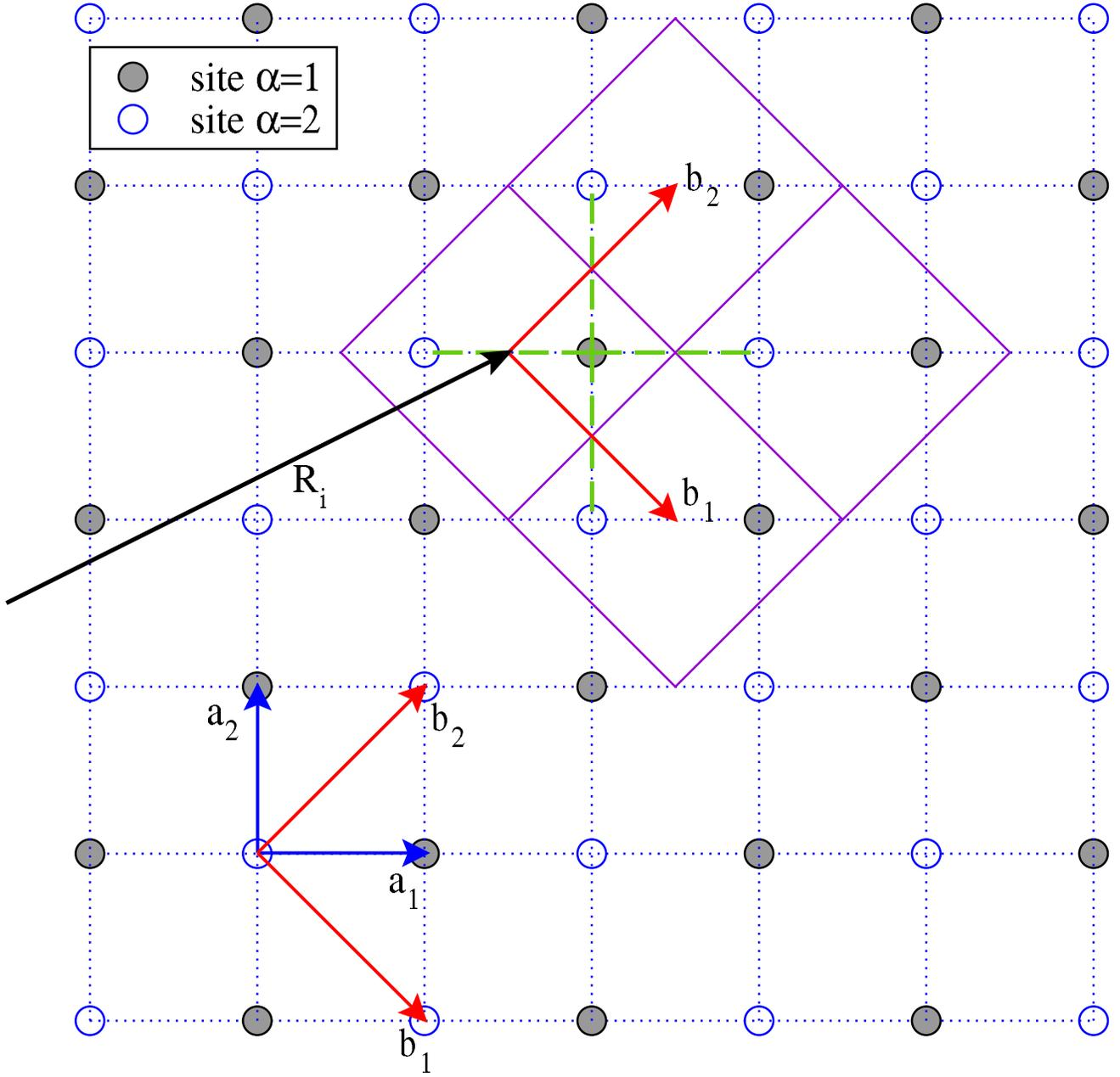
FIG. 1: Single  $(\vec{a}_1, \vec{a}_2)$  and double  $(\vec{b}_1, \vec{b}_2)$  cells for the square lattice. Nearest neighbours of  $\alpha = 1$ ,  $\vec{R}_i$  are highlighted by the green dashed lines. The four violet cells represent nearest-neighbour cells in the  $(\vec{b}_1, \vec{b}_2)$ -basis.
