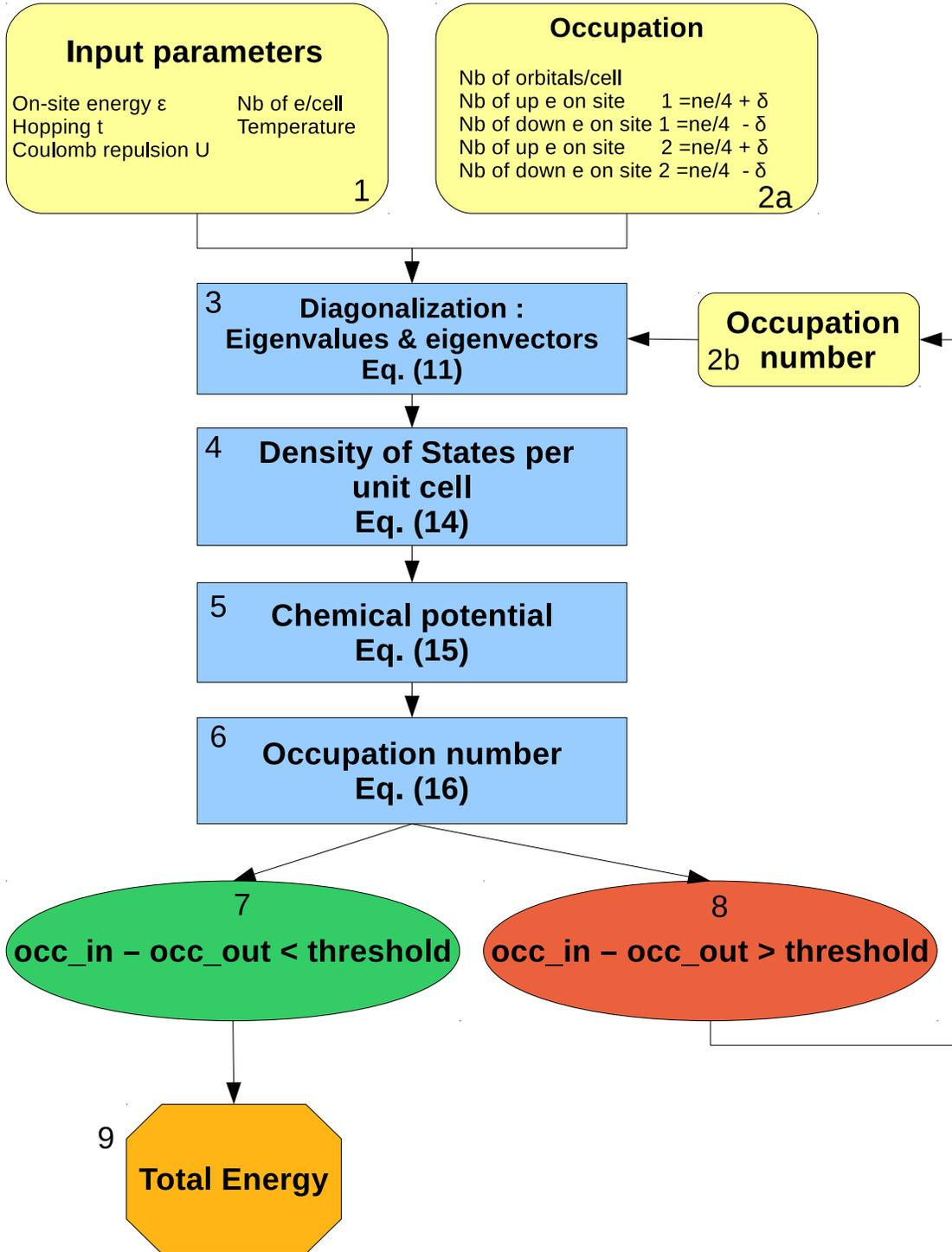
FIG. 3: Scheme of the self-consistent algorithm leading to the ground-state phase diagram of figure 6. Equations are described in the text
