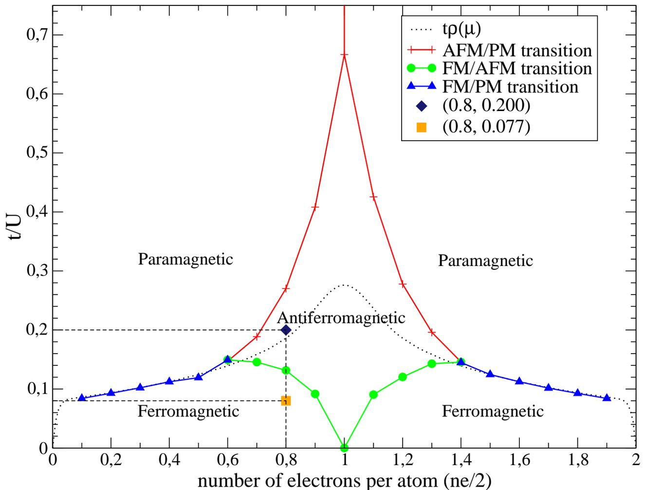
FIG. 6: Ground-state phase diagram of the Hubbard model on a square lattice as a function of the ratio  $t/U$  and of the electron filling. The physical relevance of the curve  $t\rho(\mu)$  is detailed in the text. We used an inverse-temperature value  $\beta = 0.03t$  in the equations. The two points  $(0.8, 0.077)$  and  $(0.8, 0.2)$  correspond to the band structure depicted in figure 5.
