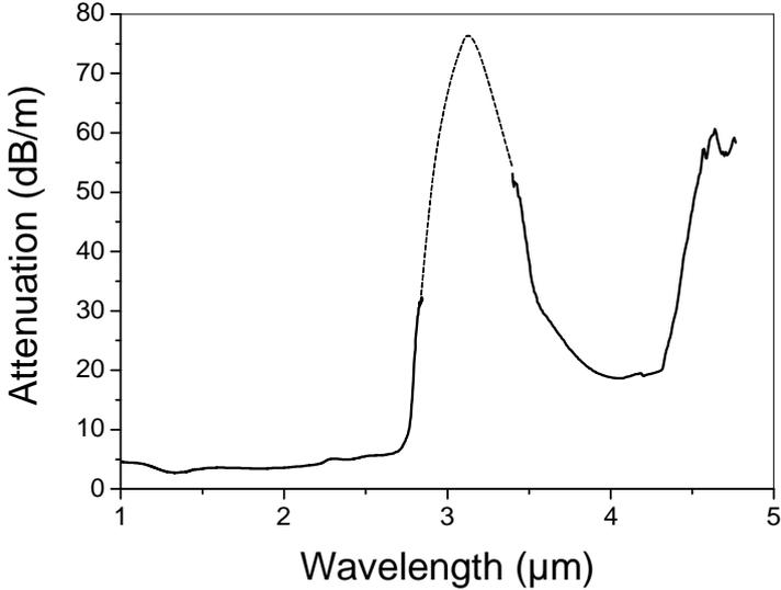
Figure 5: Attenuation curve of a Sb<sub>2</sub>O<sub>3</sub> based fiber, the dash curve concerns extrapolated points.
