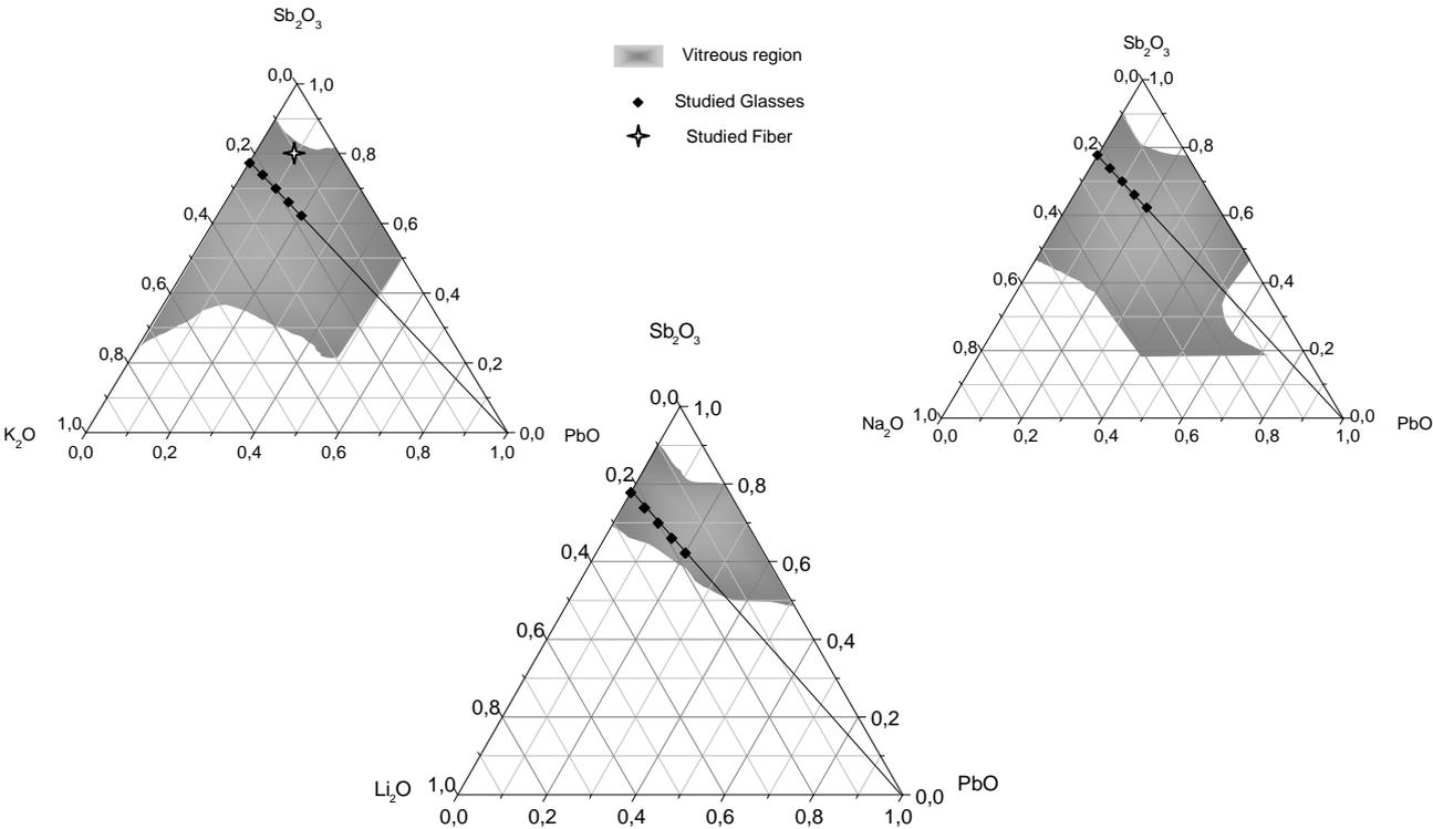
Figure 1: Sb<sub>2</sub>O<sub>3</sub>-PbO-M<sub>2</sub>O (M=Li, Na or K) glassy systems
