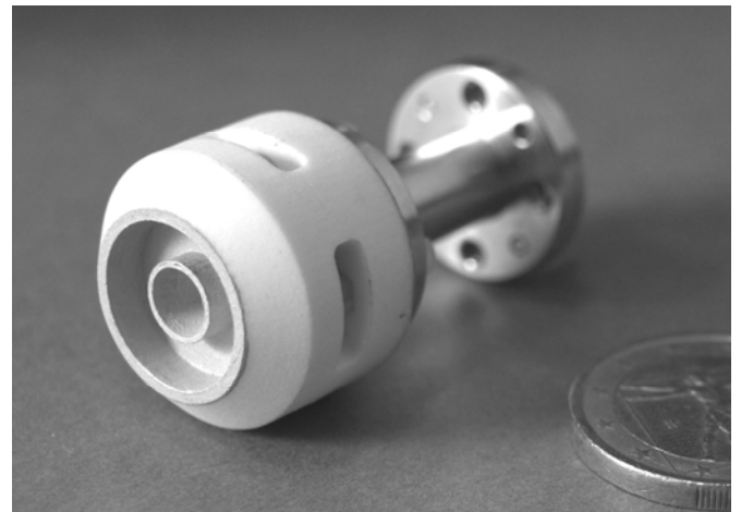
Fig. 1. Photo of the antenna prototype attached to a standard circular-to-rectangular waveguide transition. Metallized surfaces are seen in grey color.
