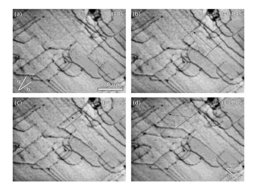
Figure 2. Motion of screw dislocations during *in situ* TEM straining; the dislocation labelled A cross-slip from (321) plane to (110) plane; a dashed line indicates the previous position of the dislocation A on each frame.
