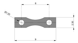
Figure 1. Dimensions of micro tensile specimens for in situ TEM experiments.
