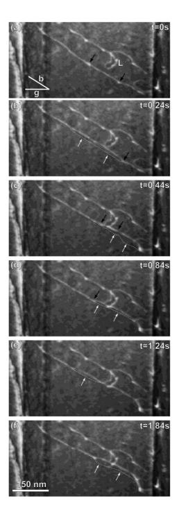
Figure 3. Weak beam dark field micrographs of screw dislocations gliding in a {112} plane taken during *in situ* TEM straining; a dashed line indicates the previous position of the moving dislocation on each frame.
