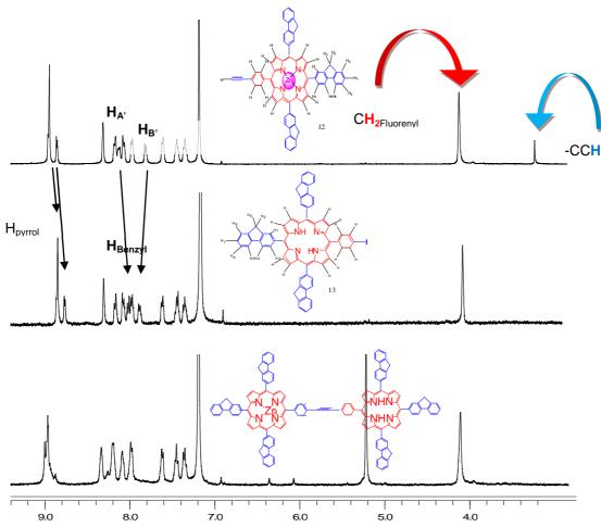
Figure 4: <sup>1</sup>H-NMR studies (in CDCl<sub>3</sub>) of Dimer 7 (with a CH<sub>2</sub>Cl<sub>2</sub> pic), in comparison to zinc porphyrin complex 12 (on the top) and for iodo porphyrin-intermediate 13 showing the shift as indicated by the arrows.
