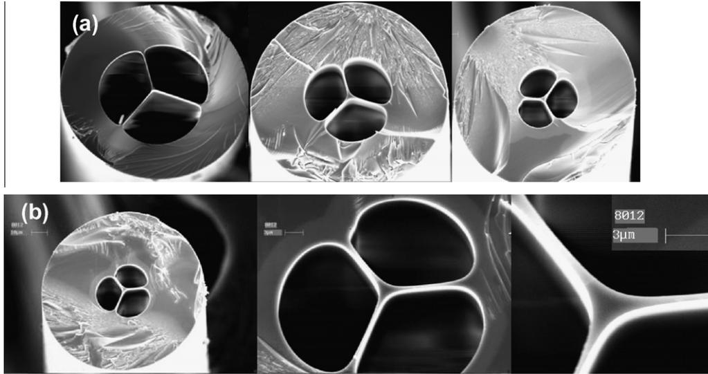
**Fig. 2.** Geometrical profiles of microstructured optical fibers drawn from preforms depicted in Fig. 1. (a) Different suspended core fibers obtained with a good control of their geometry:  $S_{\text{holes}}/S_{\text{fiber}}$ : 0.56; 0.45 and 0.35 and  $D_{\text{core}}$ : 1.6; 2.0 and 2.2  $\mu\text{m}$  respectively; and (b) SEM pictures used for the characterization of the geometrical profiles of TZN suspended core fibers.
