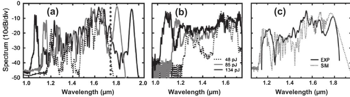
**Fig. 9.** Supercontinuum generation in a 2.2  $\mu\text{m}$  core TZN MOF for three injected pulse energies: (a) Numerical predictions and (b) experimental measurements for a 58 cm long fiber (black points: OSA spectral window limit); and (c) numerical prediction and experimental measurement (with the help of an InSb detector) for a 20 cm long fiber and a pulse energy of 80 pJ.
