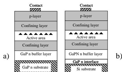
**Fig. 1:** (a), structure of the future DEL with QDs or QWs on GaP substrate. (b), structure of the DEL with QDs or QWs on GaP deposited on silicon substrate.
